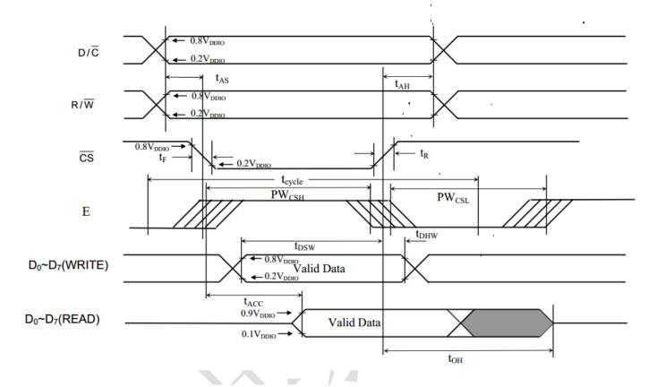
Parallel 6800-series Interface Timing Characteristics
